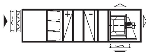
**Combined supply and withdrawn air device**
